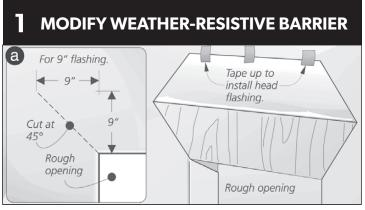
Make the following diagonal cuts at the top of the rough opening corners. Example: for 9" flashing measure as follows: 9" up and 9" over, making a 45° angle (1a). Cut on the diagonal from marked point to the rough opening corner. Gently raise the top edge of the weather-resistive barrier and tape the corners and the center to the barrier surface above. This will allow for the installation of the window and the jamb and head flashing later.
