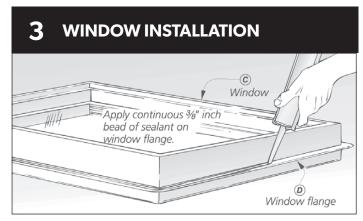
Before installing the window, apply a continuous 3/8" bead of Polymer Sealant to the backside (interior) of the mounting flange. Install the window according to the window manufacturer's instructions.
