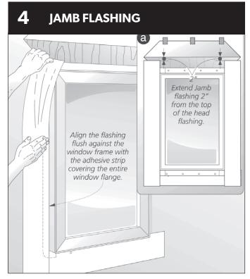
Prior to installing the jamb flashing wipe the jamb flange and weather-resistive barrier with a clean rag to ensure proper adhesion. Then cut two strips of flashing long enough to extend beyond the sill flashing and 2" below the top of the head flashing. Remove the release paper and align the flashing flush against the window frame with the adhesive strip covering the entire window flange. Follow this procedure for the other side of the window.
