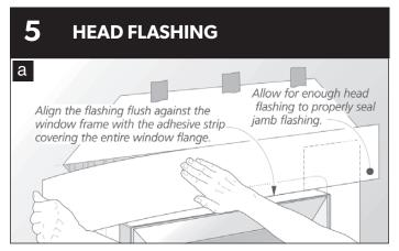
Wipe the head flange, jamb flashing, weather-resistive barrier, and sheathing with a clean rag. Cut a piece of flashing long enough to ensure that the head flashing extends a minimum 1" beyond the jamb flashing. Install the head flashing by pressing firmly in place in one direction to prevent voids.
