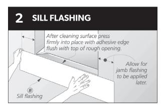
Cut the sill flashing to the width of the rough opening plus twice the flashing width. Wipe the surface of the weather-resistive barrier with a clean rag to ensure proper adhesion. Remove the release paper and press the sill flashing in place so that the edge of the flashing's adhesive is level with the top edge of the rough opening.
