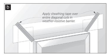
Finally, allow the flap of the weather-resistive barrier at the head to lay flat over the head flashing. Apply a new piece of sheathing tape over the entire diagonal cut made in the weather-resistive barrier and press firmly in place.
